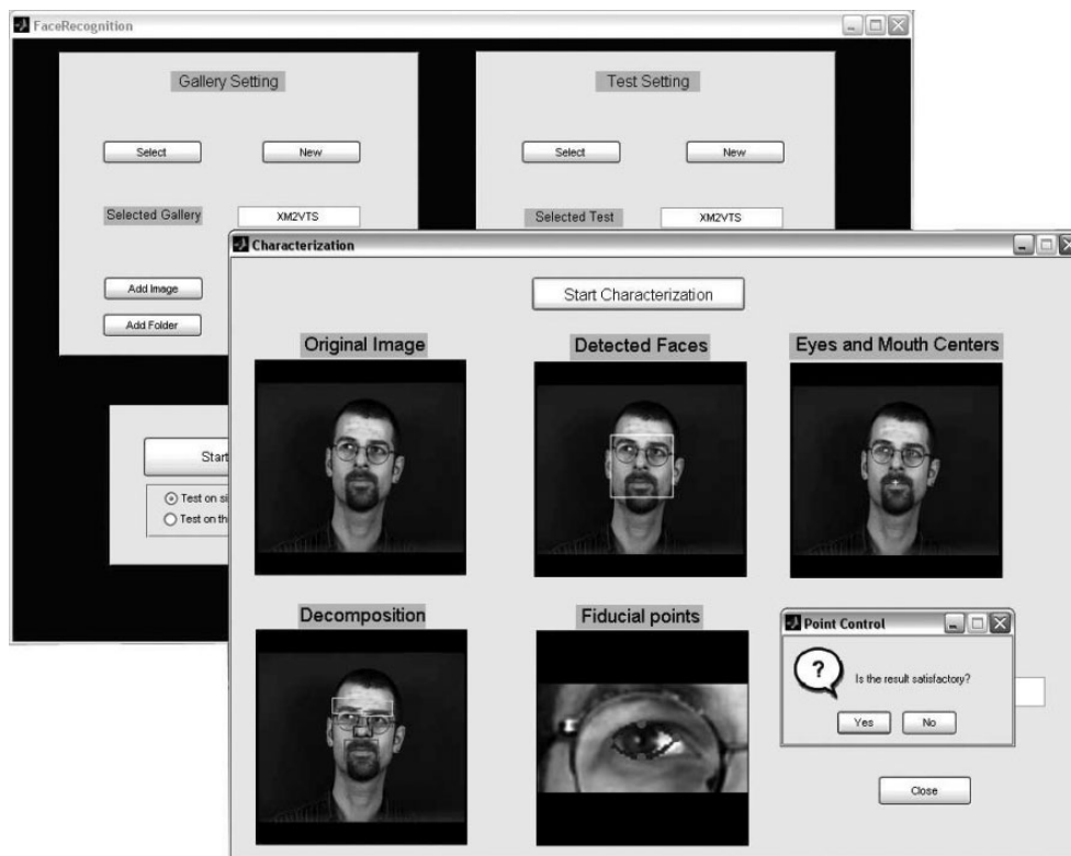
FIG. 3—A screen shot of the interactive user interface when the system is used in the assisted modality on a typical XM2VTS image.
