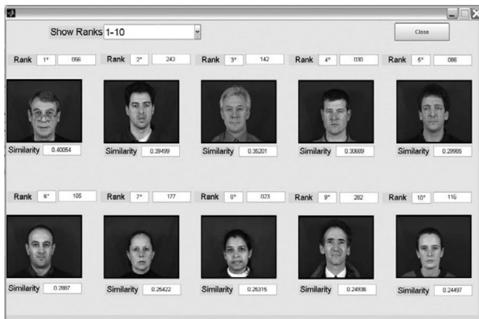
FIG. 5—This is what would pop up if the Show results button in Fig. 4 were to be pressed: the figure shows the first 10 subjects in the gallery that “resemble” the most the probe image. For every subject, it reports the gallery ID and the similarity score.
